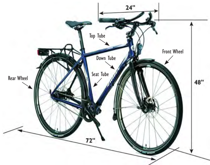
Figure 2-1: Typical bicycle dimensions
