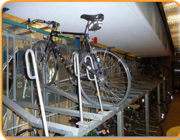
Figure 2-7: Swiveling locking arm (photo: John Ciccarelli)
