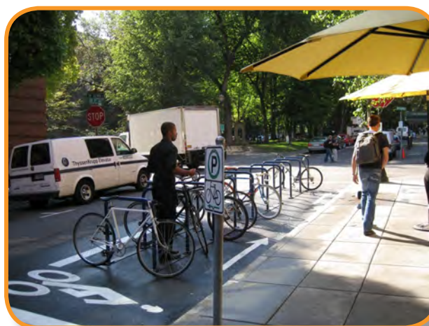
Figure 2-39: Pavement legends designate the cyclist dismount area and circulation pattern. (photo: City of Portland, Ore.)
