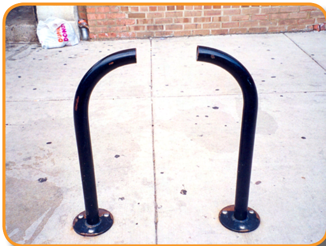
Figure 2-12: Cut round tubing rack (photo: Eric Anderson)
