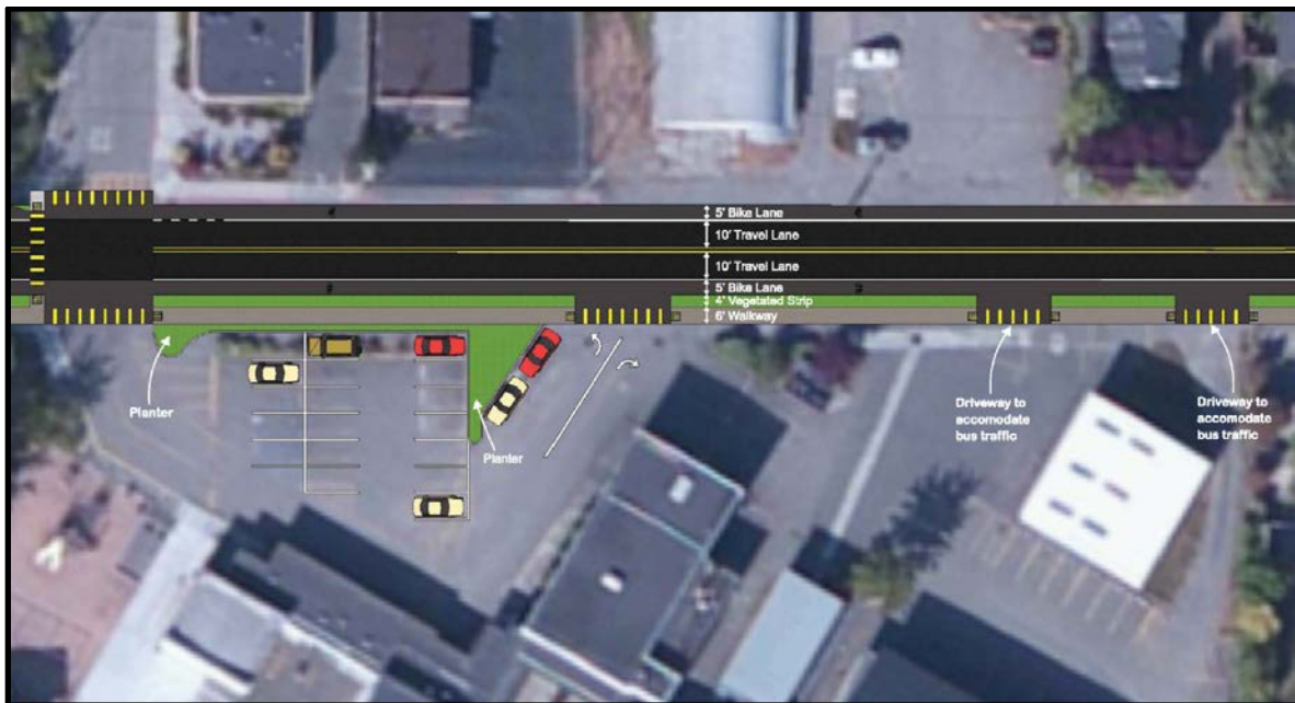
Figure 3.2 Proposed cross-section of the Jacoby Creek School Frontage with the separated path alternative stated in Alternatives One and Two (SHN et al., 2017).
