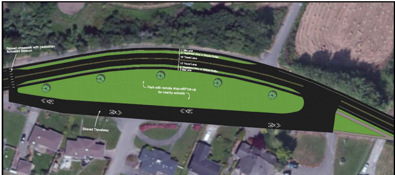
Figure 3.1 Proposed improvements to the Northern Segment where Bayside Rd. and Old Arcata Rd. meet (SHN et al., 2017).
