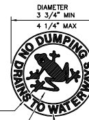
LETTERS 1/2" AQUATIC CREATURE GRAPHIC (FROG SHOWN) RECEIVING WATER BODY (WATERWAYS SHOWN) PLAN DRAINAGE INLET MARKER (MEDALLION)
