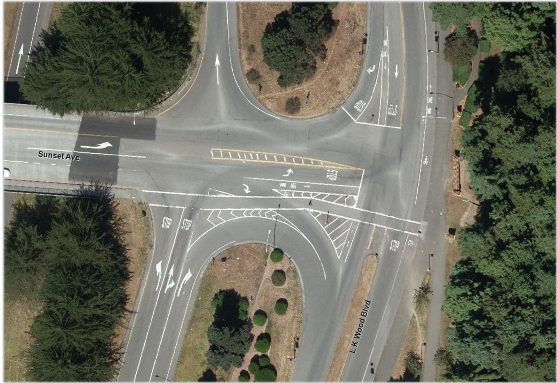
Figure 2.1 The current configuration of the two intersections located within the project area. The Sunset Avenue/US 101 northbound ramp intersection is a four-legged intersection with the north and south leg acting as US 101 Northbound on- and off- ramps. The Sunset Avenue/LK Wood Boulevard is an all-way stop located 150 feet east of the Sunset Ave/US 101 northbound ramps intersection.
