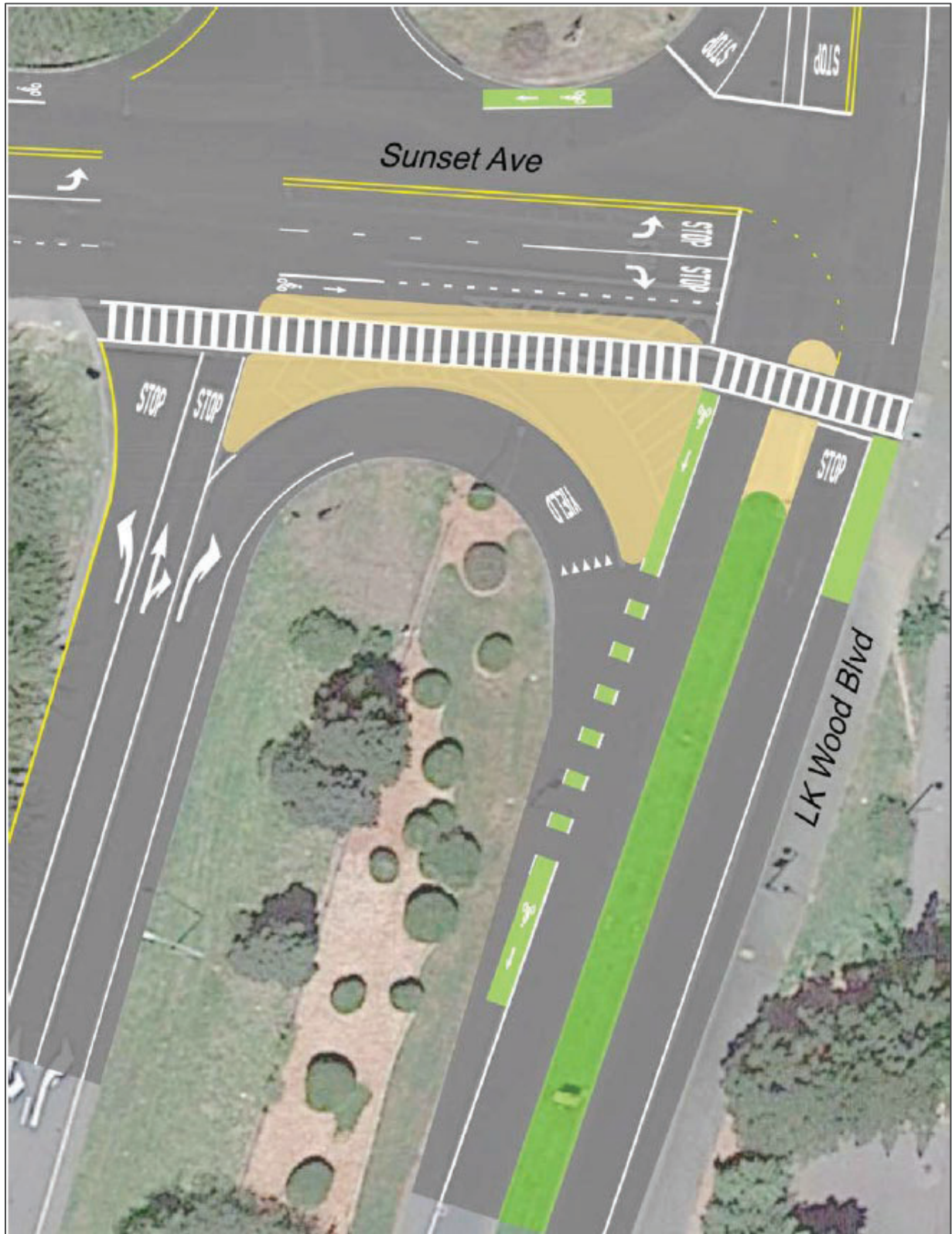
Figure 3.1 Proposed Alternative Two for the Sunset Avenue/LK Wood Boulevard project area. This alternative will provide more visible striping and install raised islands along the southern side of the project area. A right turn lane will be added to Sunset Avenue to access southbound LK Wood Boulevard.
