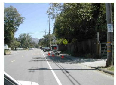
The speed trailer pictured above reminds motorists to observe the speed limit and serves as a temporary traffic calming measure in front of Redway Elementary on Whitmore Road.
